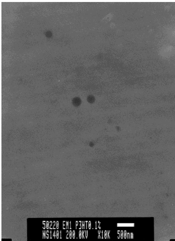
Figure 1 TEM micrograph of poly(3-hexylthiophene) P3HT in a poly(methyl methacrylate) film. The content of P3HT (no. 2) was 0.1 wt %.
